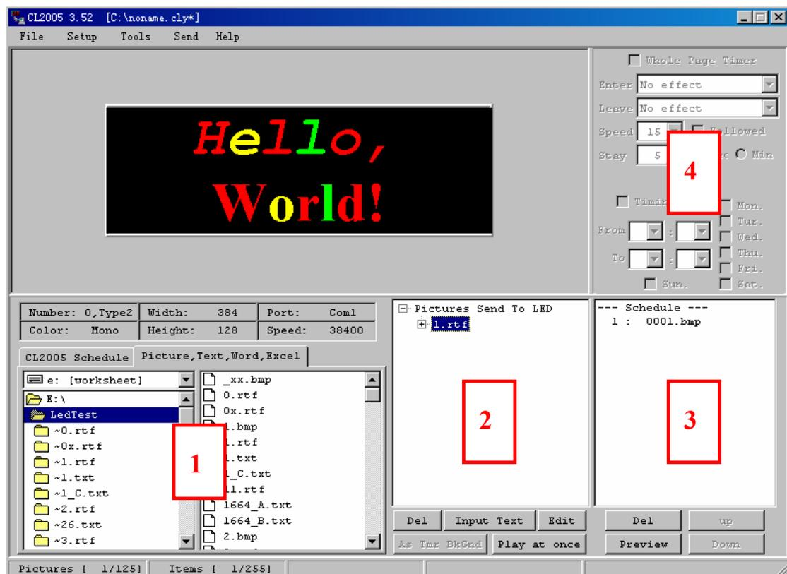
Choose the file from the window 1, double click the filename to add the file to window 2, then double click the filename in window 2 to add the file to window 3. Finally adjust the effect and
